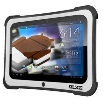
The RangerX has integrated WLAN 802.11a/b/g/n, Bluetooth 4.0, GPS and optional 4G LTE mobile broadband to keep workers connected. It has more onboard I/O than most light and compact tablets, including a USB 2.0 port, a micro USB 2.0 port, audio, and micro HDMI-out. Optional I/O ports include HDMI-in and an RJ-45 LAN jack. Other integrated features include front and rear cameras, an RFID/NFC reader, and an optional CAC reader.
